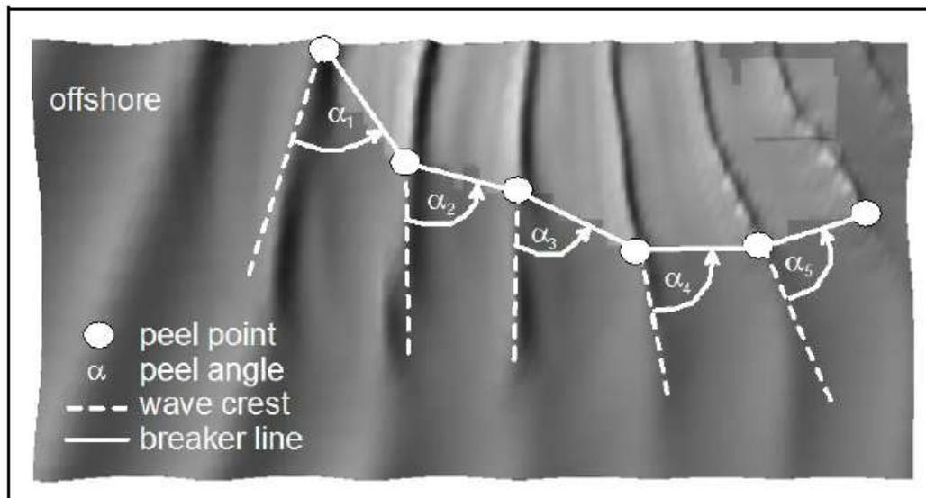
Figure 4.2: Peel angle definition (Source: Smit et al., 2007)
