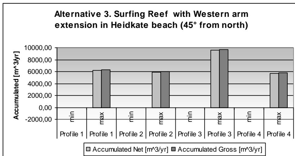
Figure 6.13: Accumulated sediment for Alternative 3 (45° from North).
