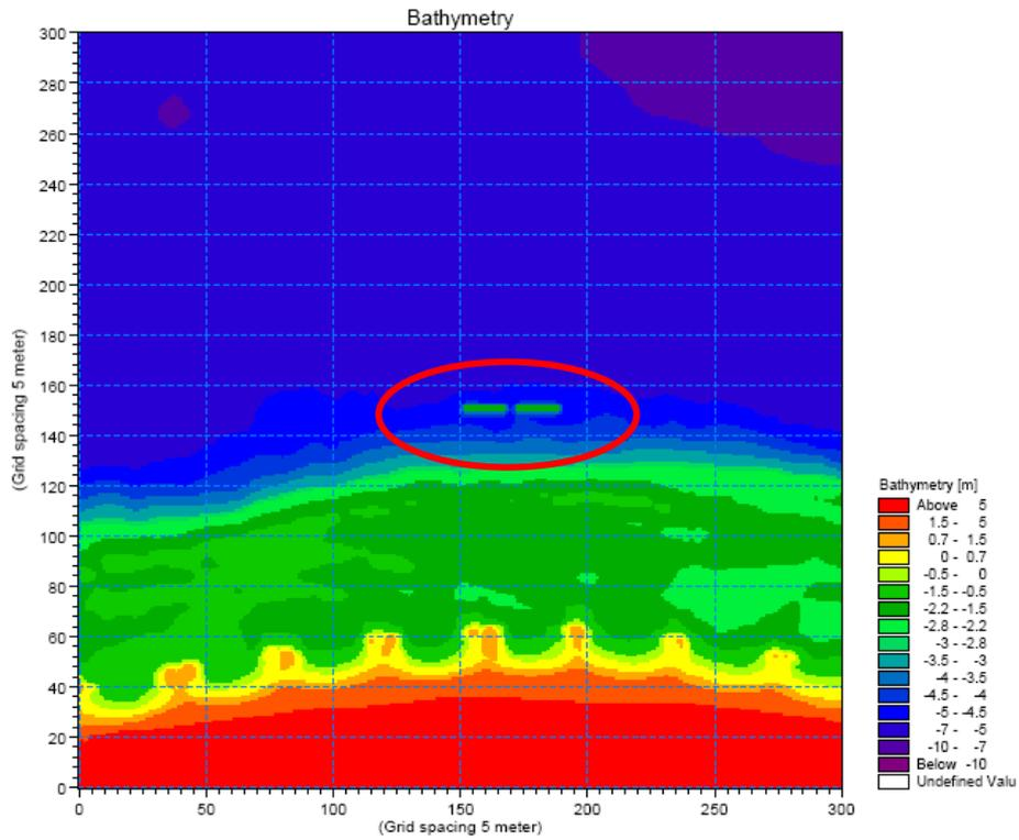
Figure 4.26: Alternative 9. Reef Ball breakwater in Heidkate Beach.
