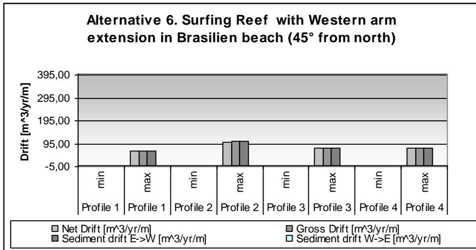
Figure 6.26: Sediment drift for Alternative 6 (45° from North).
