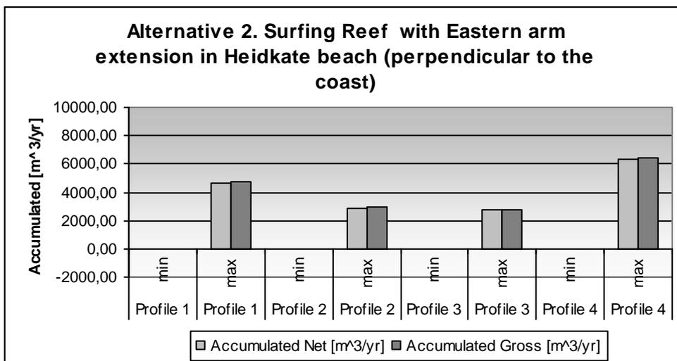
Figure 6.11: Accumulated sediment for Alternative 2 (perpendicular to the coast).
