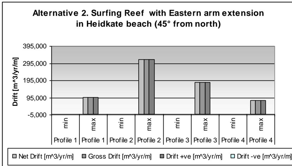
Figure 6.10: Sediment drift for Alternative 2 (45° from North).
