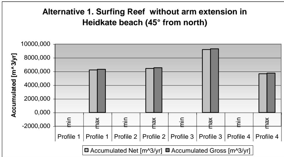
Figure 6.5: Accumulated sediment for Alternative 1 (45° from North).
