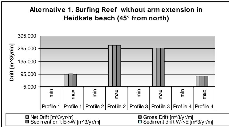
Figure 6.6: Sediment drift for Alternative 1 (45° from North).
