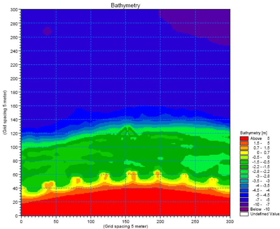
5. Artificial Reef, parallel to North and with Eastern Sleeve extension (Alternative 2)
