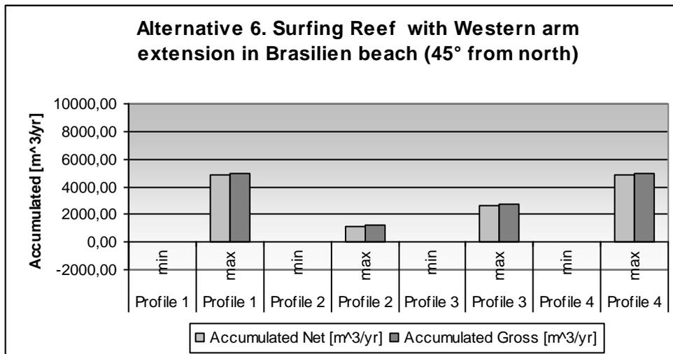
Figure 6.25: Accumulated sediment for Alternative 6 (45° from North).
