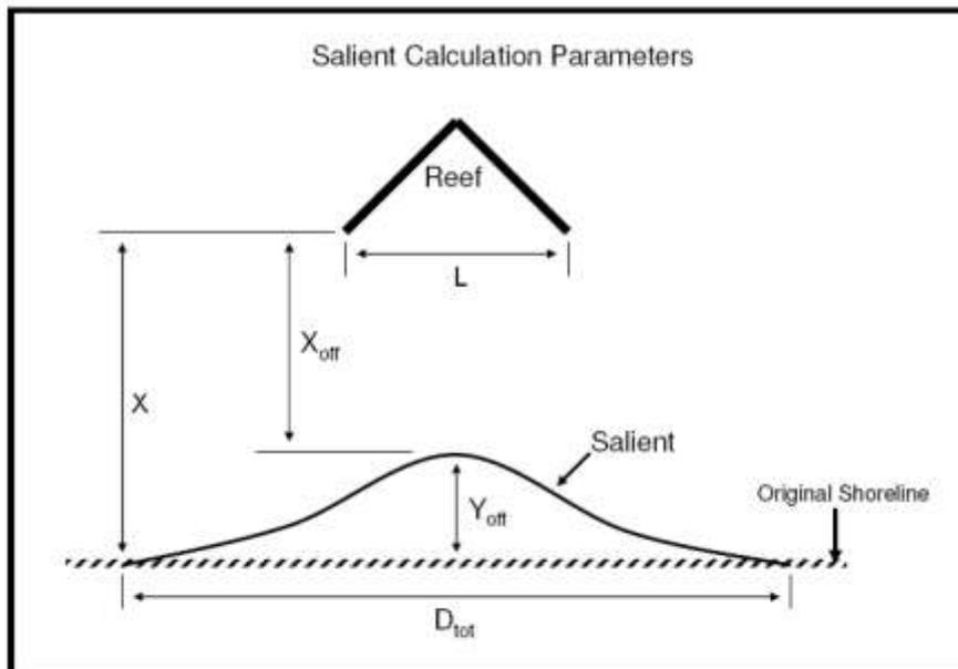
Figure 3.13: Salient calculation parameters (Source: Hearin, 2009).
