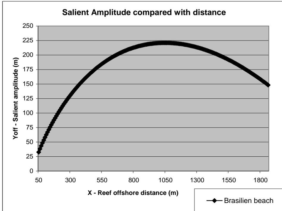
Figure 4.6: Salient Amplitude
