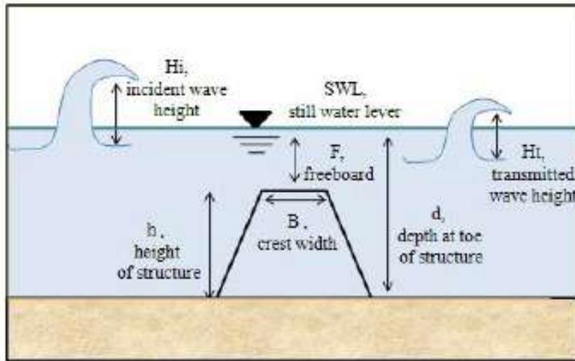
Figure 3.11: Main characteristics of submerged breakwater (Source: Arnoul, 2006).
