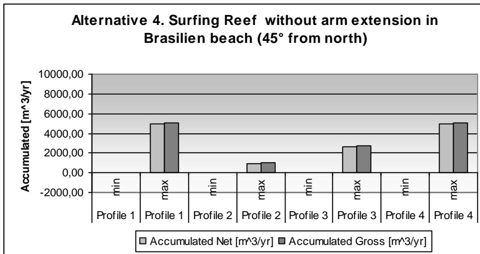
**Figure 6.17: Accumulated sediment for Alternative 4 (45° from North).**
