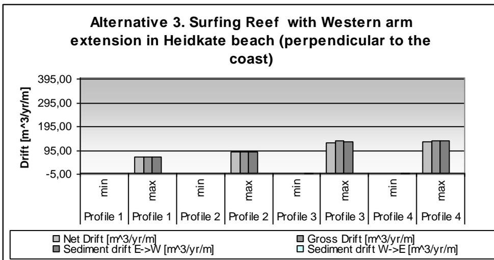
Figure 6.16: Sediment drift for Alternative 3 (perpendicular to the coast).
