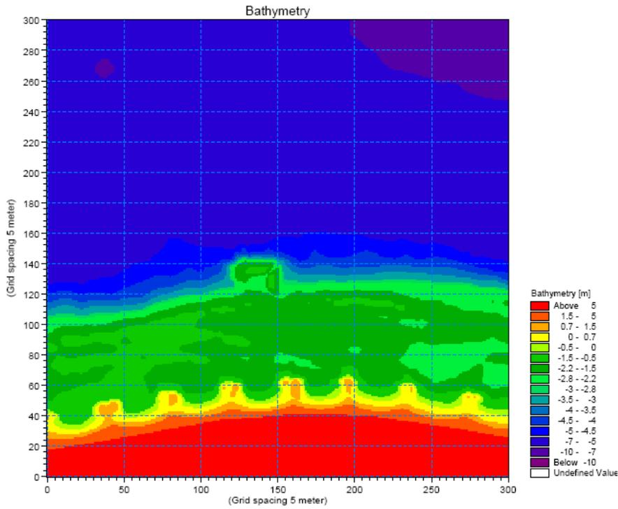
4. Artificial Reef, parallel to North and without Sleeve extension (Alternative 1)
