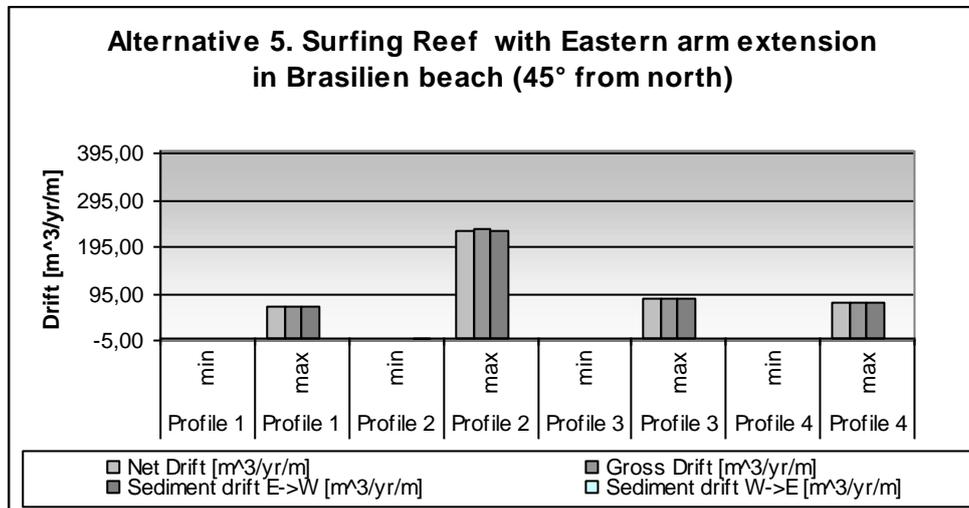
Figure 6.22: Sediment drift for Alternative 5 (45° from North).
