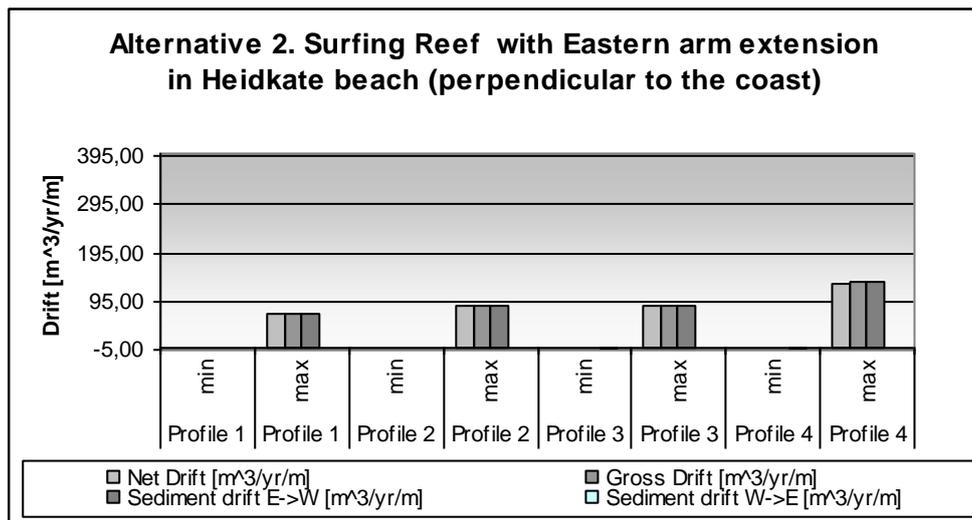
Figure 6.12: Sediment drift for Alternative 2 (perpendicular to the coast).
