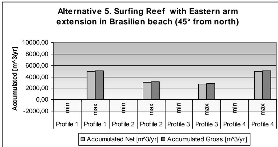
Figure 6.21: Accumulated sediment for Alternative 5 (45° from North).
