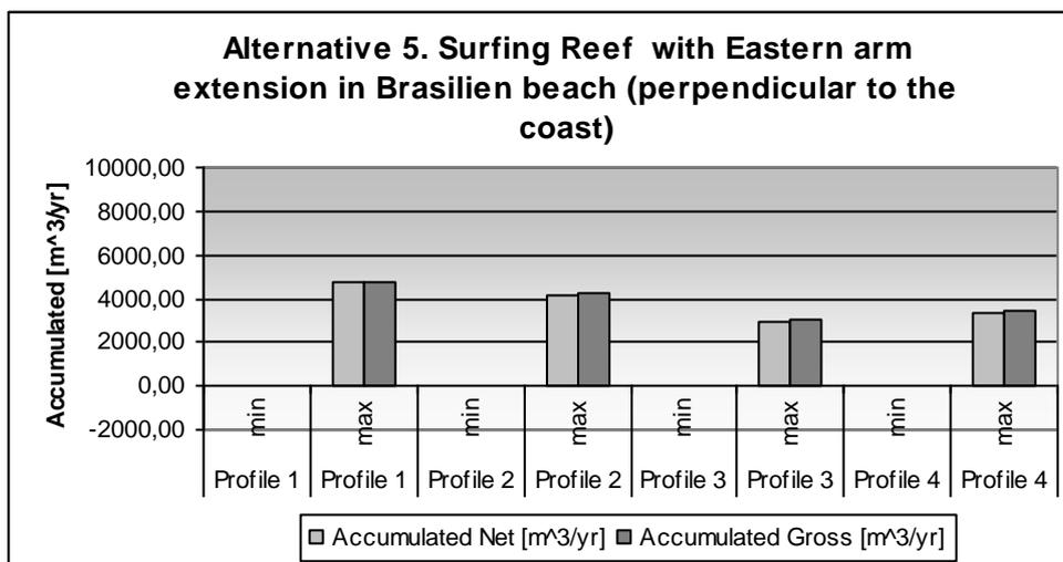
Figure 6.23: Accumulated sediment for Alternative 5 (perpendicular to the coast).
